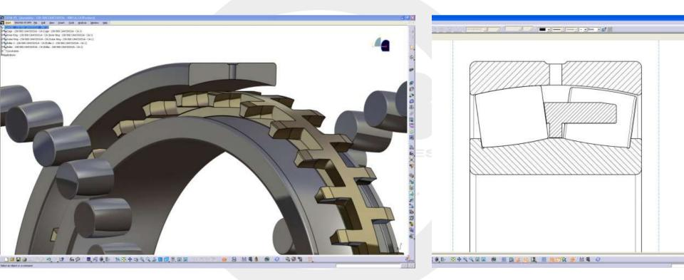
Bearing with symmetrical rollers and retaining ribs. The cage is a one-piece, double pronged machined cage of brass
