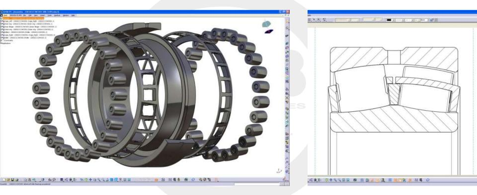
Bearing with symmetrical rollers, flangeless inner ring, a non-integral guide ring between the two rows of rollers centred on the inner ring and one pressed steel window-type cage for each roller row
