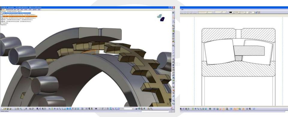
Bearing with symmetrical reinforced rollers and retaining ribs. The cage is a one-piece, double pronged machined cage of brass with separate central guide slinger
