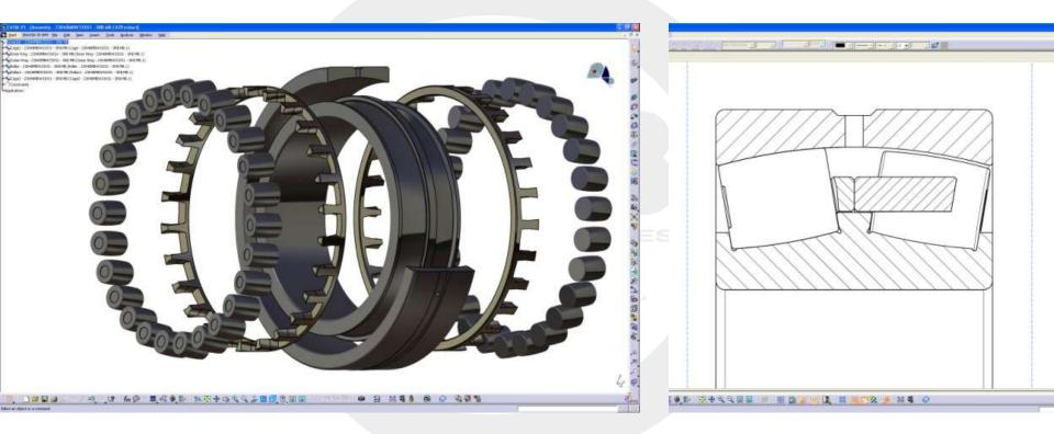
Two-piece machined brass cage guided on the inner ring central fixed rib and retaining flanges on the inner ring
