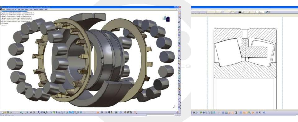
Two-piece machined brass cage guided on the outer ring and retaining flanges on the inner ring
