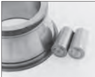
Abrasive wear Fine abrasive particle contamination.
