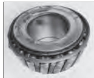
Cone large rib face deformation Metal flow from excessive heat generation.
