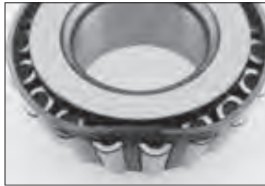
Cage deformation Improperly installed or dropped bearing.
